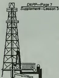
Rotary Drilling Rig
